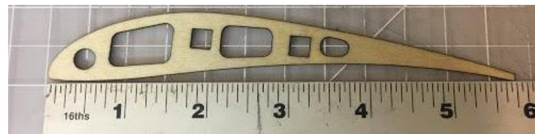
Figure 3: S1223 Airfoil shape, hole sections removed for spar location and weight reduction
