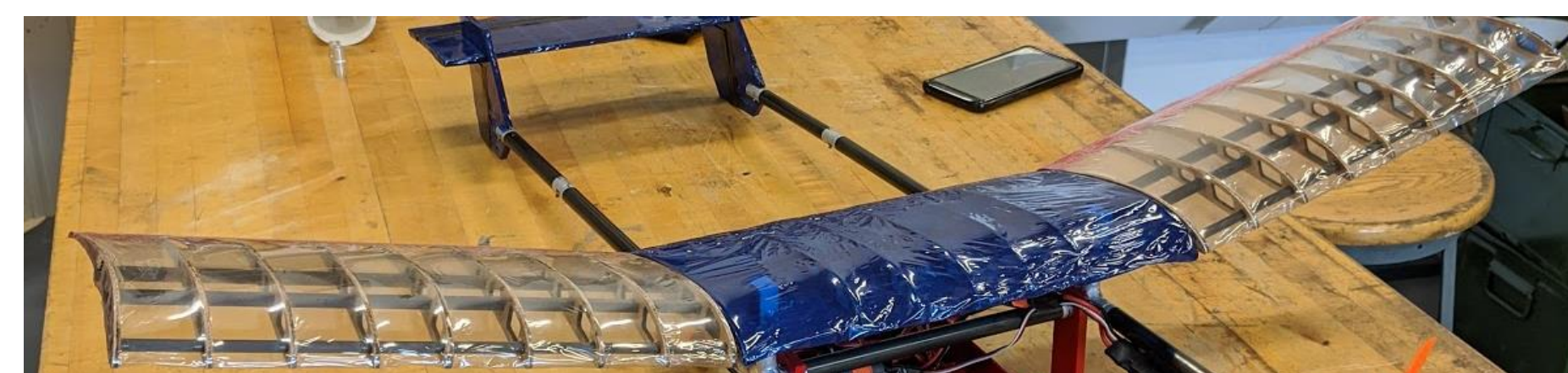
Figure 2: Dihedral U-shape of wing profile
