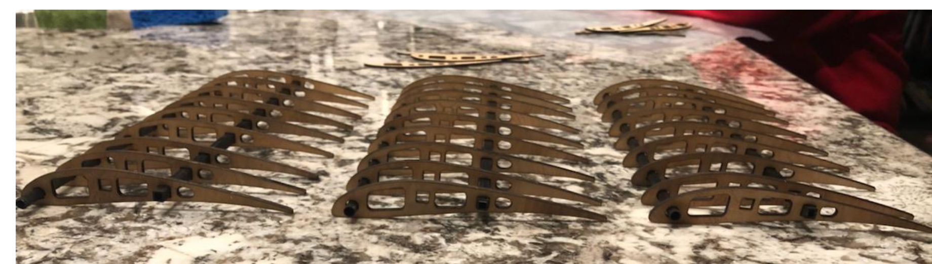
Figure 6: Wing sections under construction, prior to monokote
